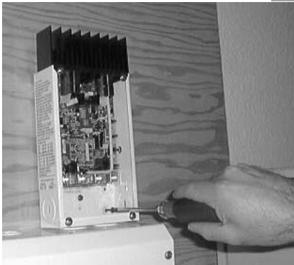
Figure 2-3 Mounting the C-Series Multifunction DC Controller
